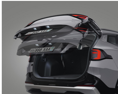
Masofadan boshqariladigan yukxona elektr yuritmasi (Smart Power Tailgate)
