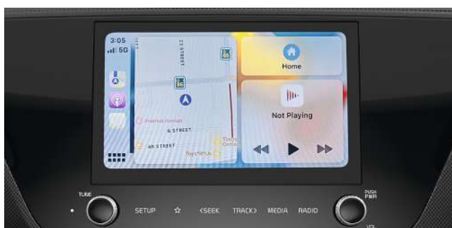
Apple CarPlay va Android Auto tizimi ishlaydigan va old panelga o'rnatilgan multimedia
